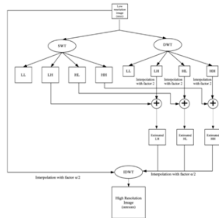
Fig3. Proposed block diagram of HWT with interpolation method
